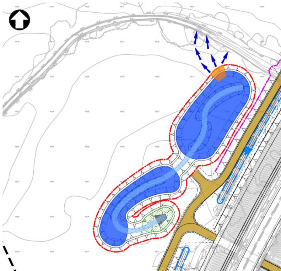
Figure 4-1: Example overland flow plan showing spillway in orange and flow path in blue
